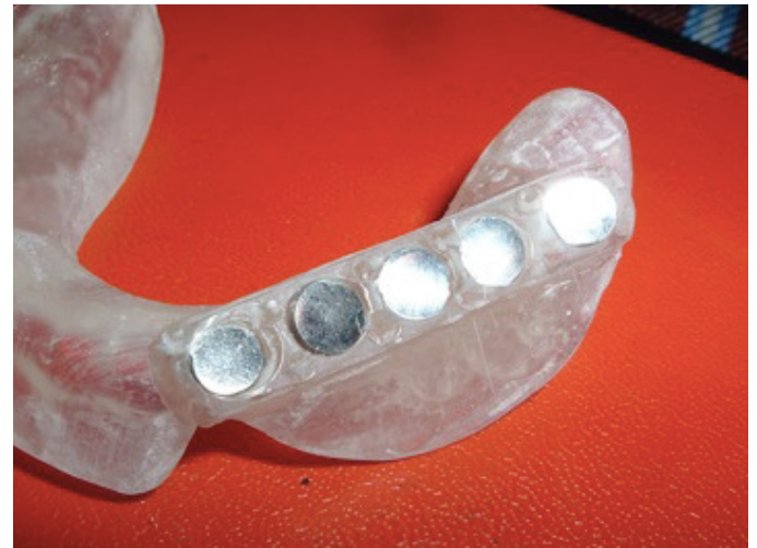
Fig. 1. Samples were placed on the trial denture to be contaminated on both sides
