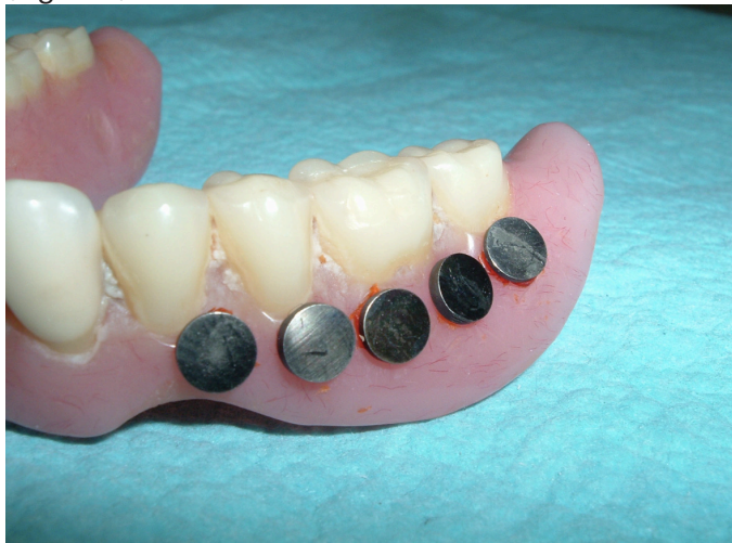
Fig. 2. Samples were attached to the right and left buccal flanges of lower denture by using self-cured acrylic resin.
