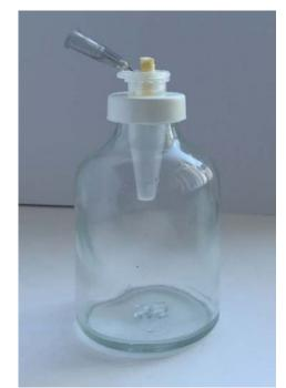
Fig. 1. The apparatus used for the collection of extruded debris.
