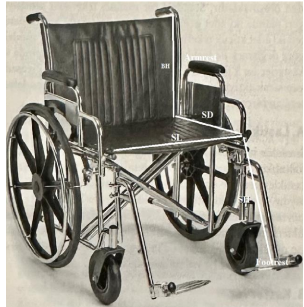
Figure 1. Picture designates the wheelchair parts. AR, armrest; BH, back height; FR, footrest; SD, seat depth, SH, seat height; SL, seat length.
