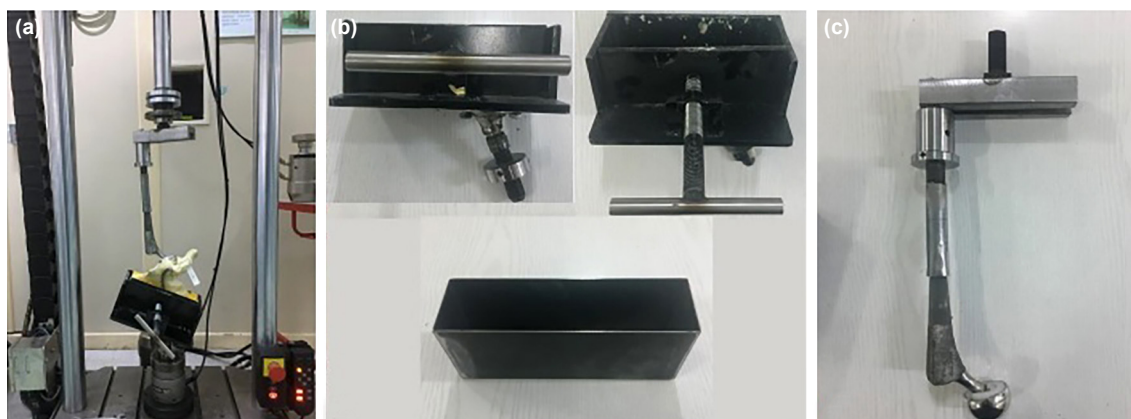
Figure 2. The experimental setup. (a) The position of the experimental setup on the Instron device. (b) Metal box setup in which bone models are embedded. (c) Femoral stem and head providing load transmission to the acetabular.
