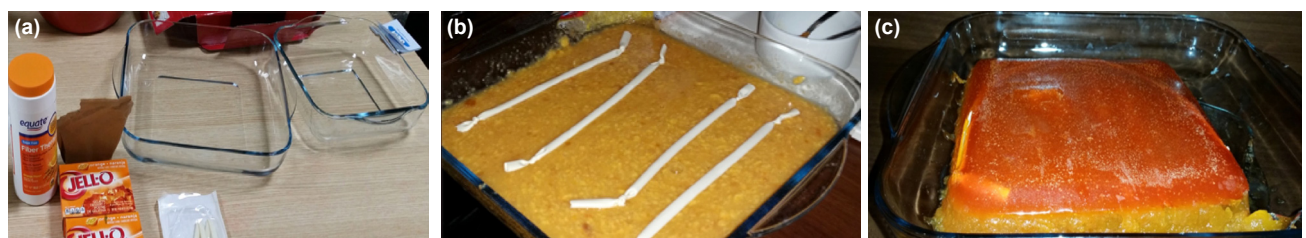
Figure 1. Preparation of a homemade ultrasound phantom. (a) Materials (tray, gelatin, psyllium, and Penrose drains) needed for the preparation of the ultrasound phantom. (b) Penrose drains are containing tap water (simulating peripheral veins) and gelatin-psyllium mixture to prolong its shelf life. (c) Penrose drains were covered on the top and bottom layers of the by gelatin-psyllium mixture.
