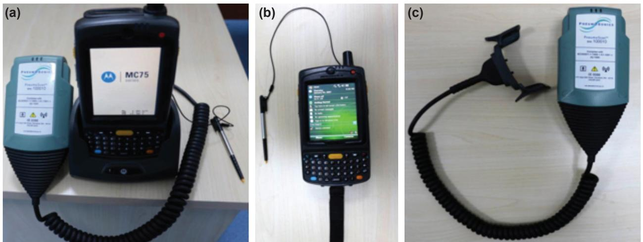
Figure 1. (a) Pneumoscan device. (b) Handheld computer. (c) MIR transceiver.
