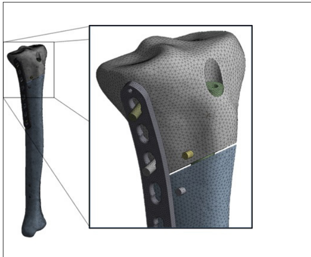
Figure 2. The biomodel meshed using tetrahedral elements.
