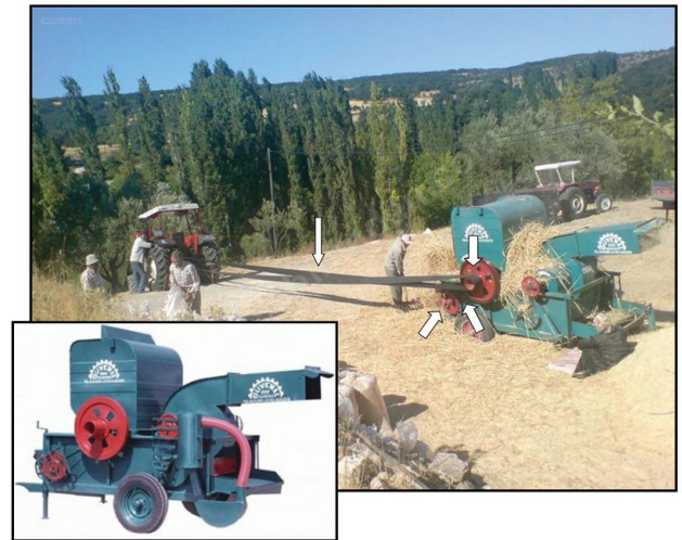
Fig. 1. The threshing machine. The arrows indicate the parts of the machinery responsible for injuries.
