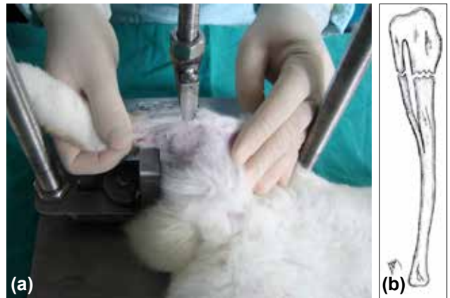
Figure 1. (a) Placement of right tibia on the apparatus. (b) Diagrammatic representation of the fracture.
