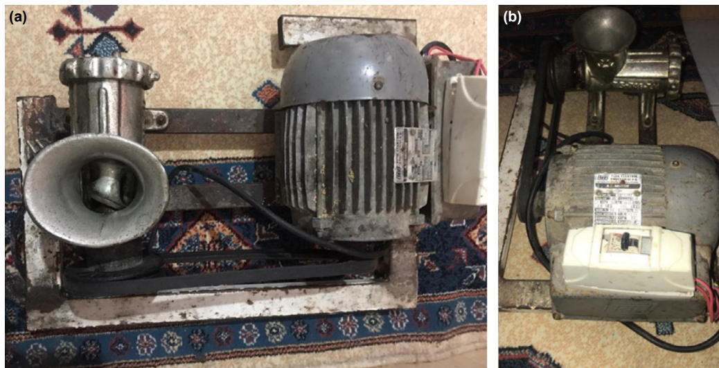
Figure 1. (a, b) Household meat grinder converted from the industrial type with the addition of an electric motor.
