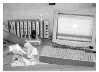
Fig. 1. BIOPAC MP 100 general EMG recording system.
