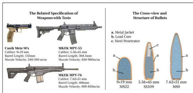
**Figure 5.** Specifications of the weapons and cross-sectional views and structures of the bullets used in the test fires.
