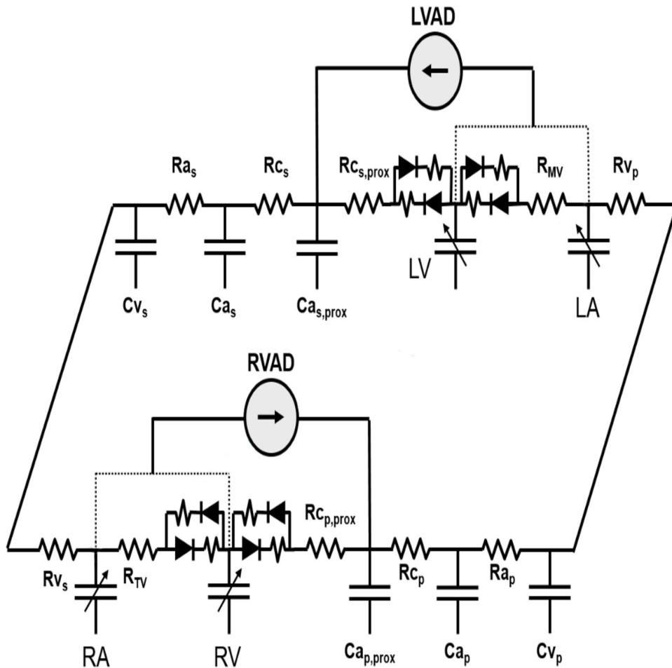
Harvi is a hemodynamic model wherein the cardiovascular system is modeled using an electrical analog as shown above. Ventricular and atrial pump features were represented by alterations of the time-varying elastance ( $E[t]$ ) theory that relates time-varying ventricular pressure ( $P[t]$ ) to time-varying ventricular volume ( $V[t]$ ). Each cardiac chamber is modeled as follows:
