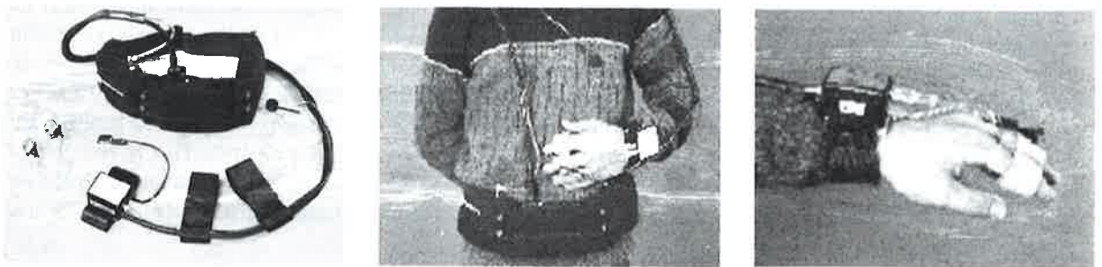
Figure 1: Portable ABPM device for continuous readings up to 24 hours with finger cuff principle. After a certain duration, usually 10 minutes, the cuff pressure changes from finger.
