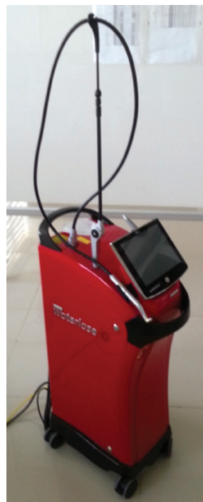
Fig. 2. Er, Cr: YSGG laser (MZ5 tip, 3.5 W, 100% water, 100% air, 20 Hz, H mode) was used to open retro cavity and to occlude dentinal tubules (MZ6 tip, 0.50 W, 0% water, 0% air, 20 Hz, H mode).
