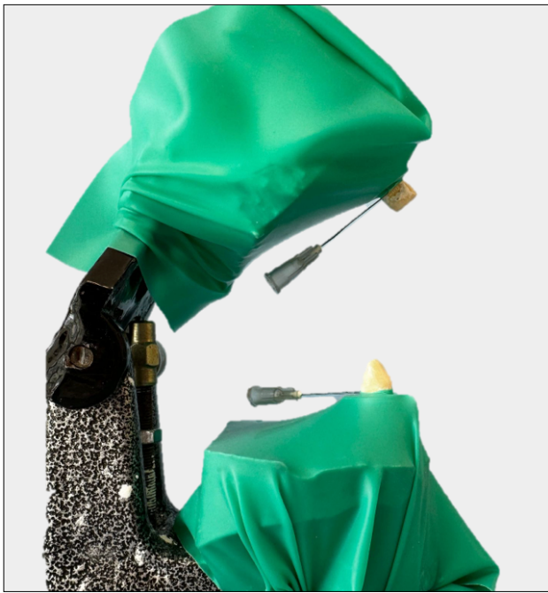
Fig. 2. Maxillary and mandibular positioning of the tooth at the experimental setup.
