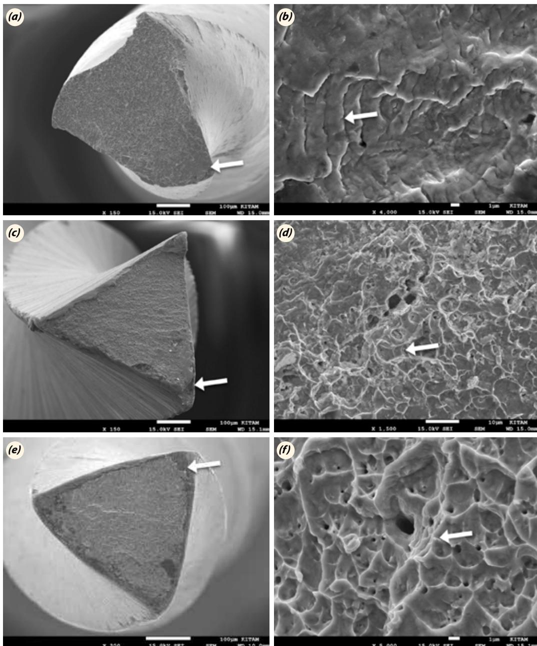
**Fig. 1.** SEM appearances of the HyFlex CM, Typhoon Cm and EdgeFile X3 files after cyclic fatigue testing. A-C-E: General view of EdgeFile X3 (a), HyFlex CM (c) and Typhoon CM (e) instrument B-D-F: High-magnification view EdgeFile X3 (b), HyFlex CM (d) and Typhoon CM (f) instrument showing fatigue striations typical of cyclic fatigue.
