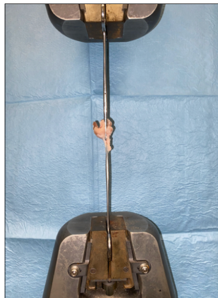
Figure 5. Placement of the dissected Achilles tendon into the tension testing device.
