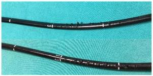
Figure 1: Surface tears on the bronchoscope
