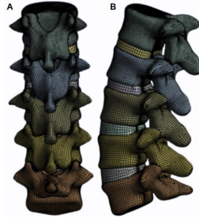
Figure 4. The mesh model of the L1-L5 spine from (A) posterior view and (B) lateral view.
