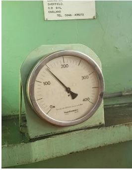
Figure 21. Tonnage gauge on the swage autofrettage plant.
