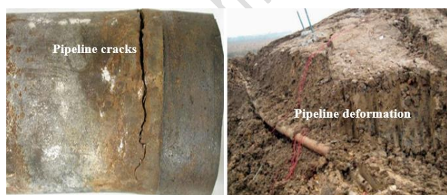
Figure 5. Typical forms of pipeline cracks [73] and deformation [54].
