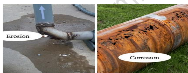
Figure 3. Typical forms of pipeline erosion [36] and corrosion [37].
