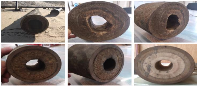
Figure 4. Typical form of pipeline scale deposit [47].
