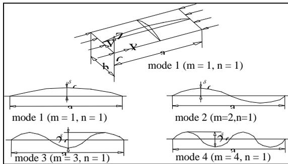
Figure 2. Plate geometry and assumed mode shapes of initial out-of-flatness
