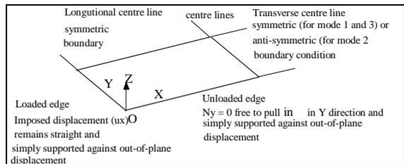
Figure 3 Boundary conditions of a quarter of a plate
