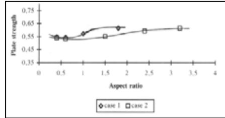
Figure 9. Variation of plate strength against aspect ratio for  $\beta = \frac{b}{t} \sqrt{\frac{\sigma_0}{E}} = 1.92$ ,  $\delta_0 = 0.1t\beta^2$  ase 1 (mode 1 + 3 and Case 2 (mode 2 + 4) Plates
