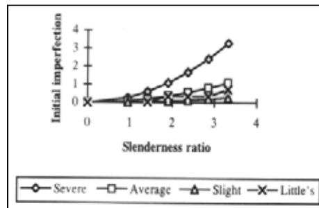
Figure 1. Initial imperfections (Severe, Average and Slight levels are assumed by Smith et al., 1987)
