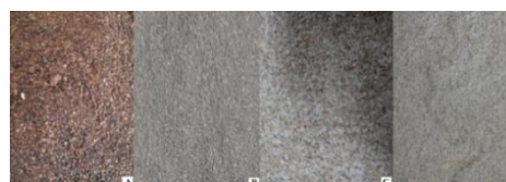
Figure 1: Used lignocellulosic fillers (a): olive pirinas, (b): 60 mesh olive pirinas flour form, (c): Turkish red pine, (d): 60 mesh Turkish red pine flour form.
