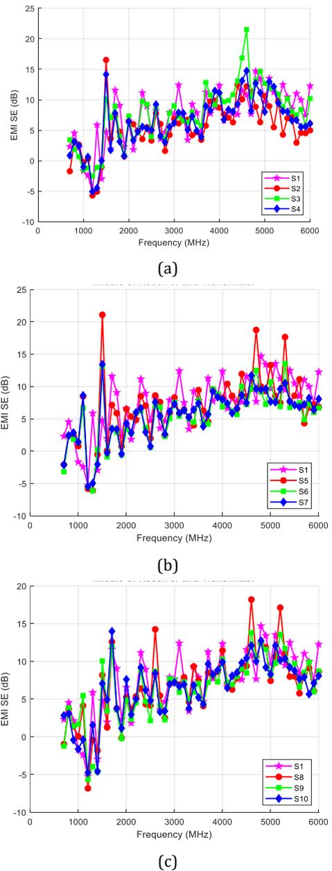
**Figure 5.** EMI SE values for CFRP composites (a)  $Fe_2O_3$  (325 mesh), (b)  $Fe_2O_3$  (50 nm), and (c)  $FeO(OH)$  in the M position
