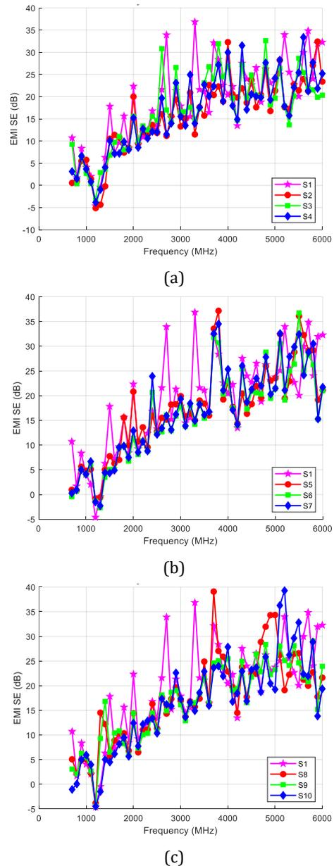
**Figure 7.** EMI SE values for composites (a) Fe<sub>2</sub>O<sub>3</sub>(325), (b) Fe<sub>2</sub>O<sub>3</sub> (50 nm), and (c) FeO(OH) in the R position.
