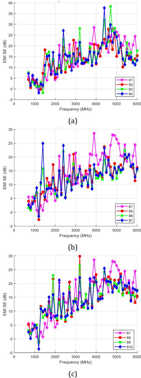
**Figure 6.** EMI SE values for CFRP composites (a) Fe<sub>2</sub>O<sub>3</sub> (325 mesh), (b) Fe<sub>2</sub>O<sub>3</sub> (50 nm), and (c) FeO(OH) in the L position
