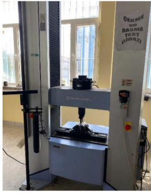
Figure 5. Shimadzu AG-X 250 kN model universal tensile-test machine
