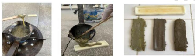
Figure 1. The melting process of waste toys
