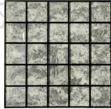
Figure 2. White and red rust rate identification for the FC sample via the template method.
