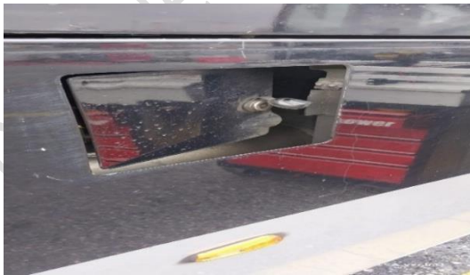
Figure 12. Damage image of the bracket from the first design during application.
