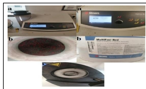
Figure 2(a): Hot molding device. (b): Phenolic resin. (c): Placing the cut sample into the hot molding chamber.
