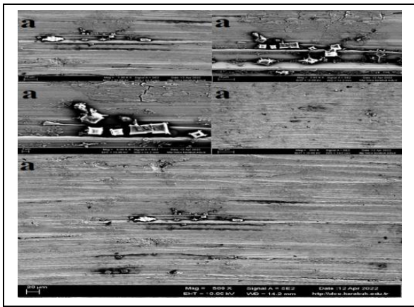
Figure 15. Ankara 10 N-1.00kx, 2.50kx, 5.00kx, 250x, 500x SEM images of the samples after the abrasion test, respectively.
