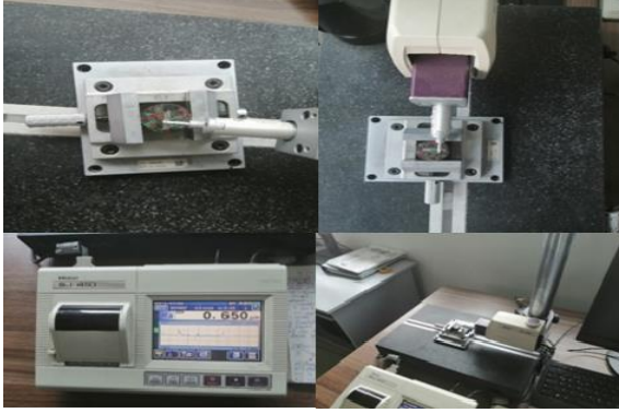
Figure 12. Placing the samples in the device for abrasion scar depth.
