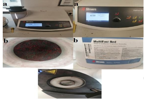
Figure 2. (a) Hot molding device. (b) Phenolic resin. (c) Placing the cut sample into the hot molding chamber.
