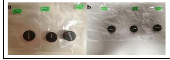
Figure 7(a): Images of samples coming out of the abrasion tester after applying 10 N, 20 N and 30 N loads to Ankara samples, respectively. (b): Images of samples coming out of the abrasion tester after applying 10 N, 20 N and 30 N loads to Gaziantep samples, respectively.
