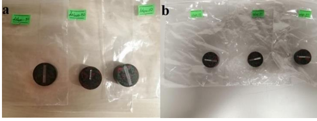
Figure 7. (a) Images of samples coming out of the abrasion tester after applying 10 N, 20 N and 30 N loads to Ankara samples, respectively. (b) Images of samples coming out of the abrasion tester after applying 10 N, 20 N and 30 N loads to Gaziantep samples, respectively
