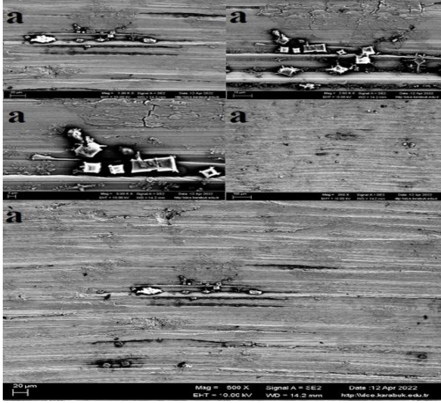
Figure 15. Ankara 10 N-1.00kx, 2.50kx, 5.00kx, 250x, 500x SEM images of the samples after the abrasion test, respectively.
