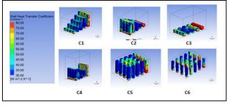
Figure 11(a). Average wall heat transfer coefficient values (C1 - -C6).
