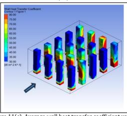
Figure 11(c). Average wall heat transfer coefficient values (*C*6).
