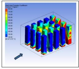
Figure 11(b). Average wall heat transfer coefficient values (*C*5).
