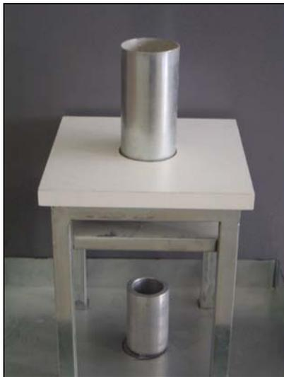
Figure 1. Uncompacted void content apparatus.
