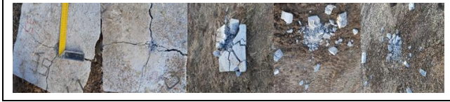
Figure 14. Contact explosion of 266,399,532,665,798 gr TNG explosives, respectively, on unreinforced plates.
