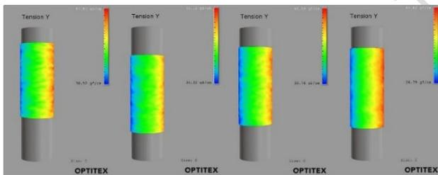
Figure 3. Tension distribution on fabric surfaces
