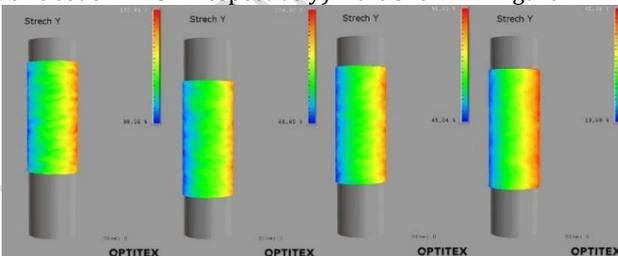
Figure 4. Stretch distribution on fabric surfaces
