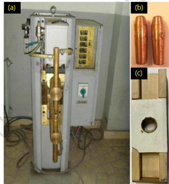
Figure 1. Experimental set-up a) RSW machine b) Electrodes c) Wooden fixture [6].
