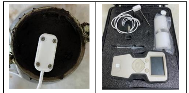
Figure 7. TEMPOS thermal properties analyzer.
