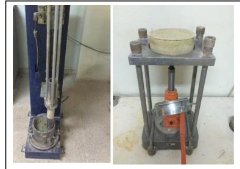
Figure 6. Standard proctor test equipment.
