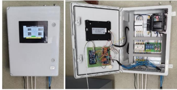
Figure 3. Data acquisition and control panel.
