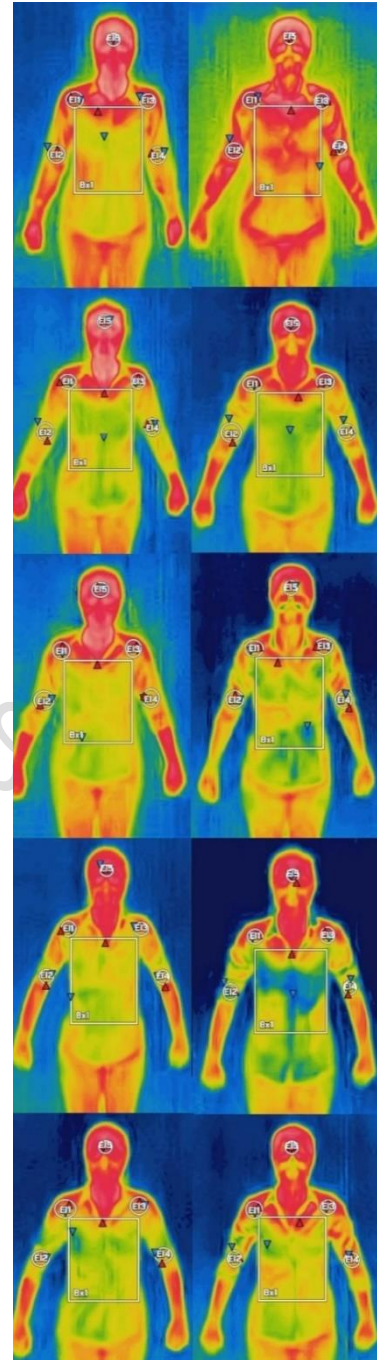
Figure 13 The thermal imaging of subject before and after activity in wear-trials respectively (1-2-3-4-5).
