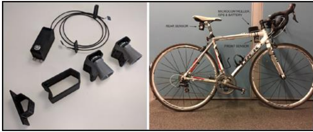
Figure 9. Dual ultrasonic distance meters mounted on bicycles for the study [64].
