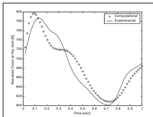
Figure 4. Comparison of an experimental and a theoretical force resultant for the hip joint
