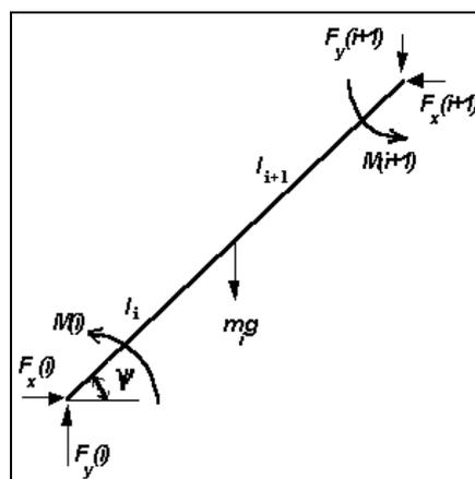
Figure 1. A typical rigid link in an  $n$ -link open chain mechanism
