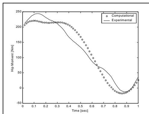
Figure 3. Comparison of an experimental and a theoretical moment change for the hip joint
