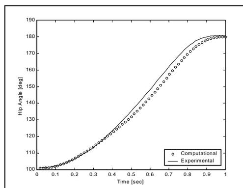
Figure 2. Comparison of an experimental and a theoretical motion trajectory for the hip joint
