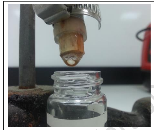
Figure 2. View of the filter placed in the filtration module under operation
