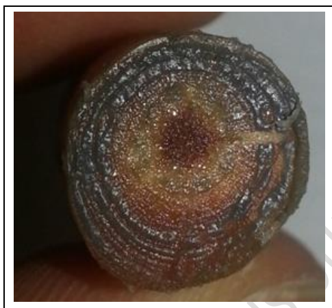
Figure 3. Cake layer formation on the filter surface (stone pine)
