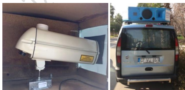
Figure 8. Average speed cameras setup placed on the vehicle (average speed camera&camouflage within luggage) [43],[65].
