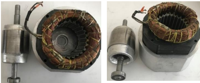
Figure 9. Prototype model of the stator and rotor of SPIM (a) Front view and (b) Side view
