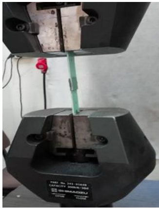
Figure 4. Performing of lap shear tests on tensile test machine
