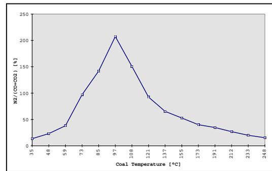
Figure 3. Changes in N<sub>2</sub>/(CO+CO<sub>2</sub>) with Temperature (Morris, 1988)
