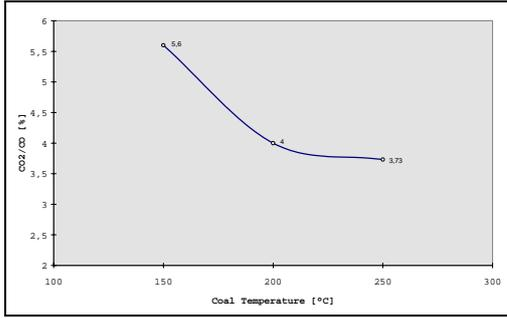
Figure 2. Changes in CO<sub>2</sub>/CO with temperature (Morris, 1988)
