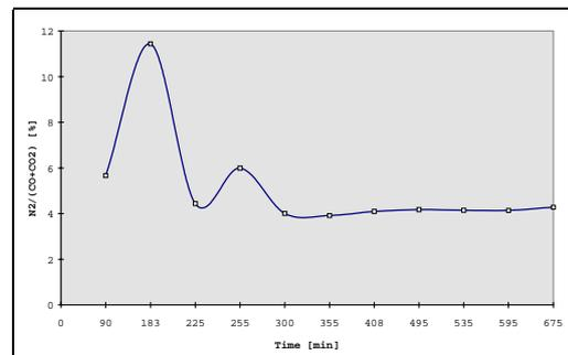
Figure 4. Changes in N<sub>2</sub>/(CO+CO<sub>2</sub>) with time (Morris, 1988)
