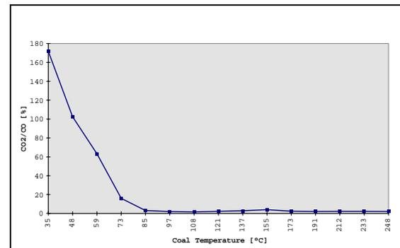
Figure 1. Changes in CO<sub>2</sub>/CO with temperature (Morris, 1988)
