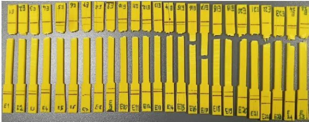
Figure 7. Specimens fractured after tensile test.
