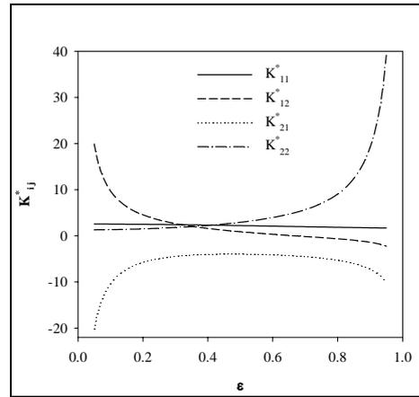
Figure 8. Dimensionless stiffness coefficients for short circular bearing
