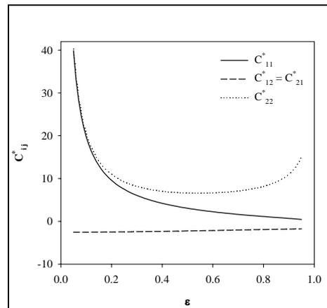
Figure 9. Dimensionless damping coefficients for short circular bearing
