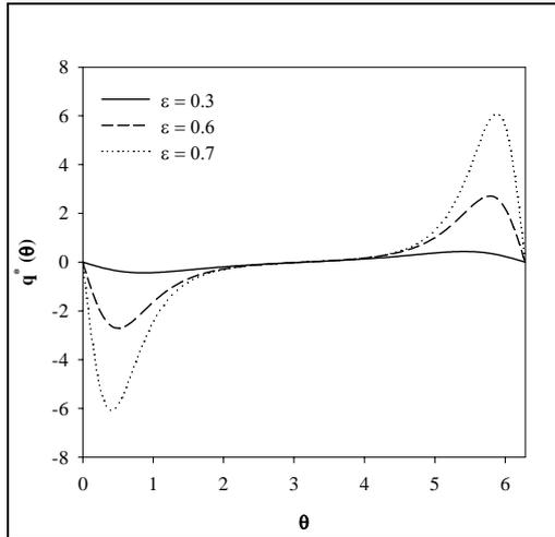
Figure 4. Fluid film force per unit length in the circumferential direction for several values of  $\varepsilon$
