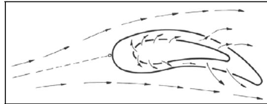
Figure 1. The cooling of a turbine blade by impingement air jet
