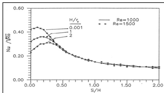
Figure 6. Non-dimensional heat transfer coeff. (Re = 1000, 1500)
