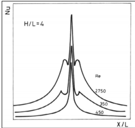
Figure 2. Variation of local heat transfer coefficients between a plate and impinging two dimensional air jet (Gardon ve Akfirat, 1966)
