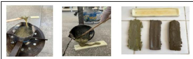
Figure 1. The melting process of waste toys.
