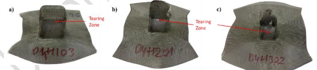
Figure 13. Results of the deep drawing process using various drawing depths; a) 30, b) 40, c) 50 mm drawing depths.
