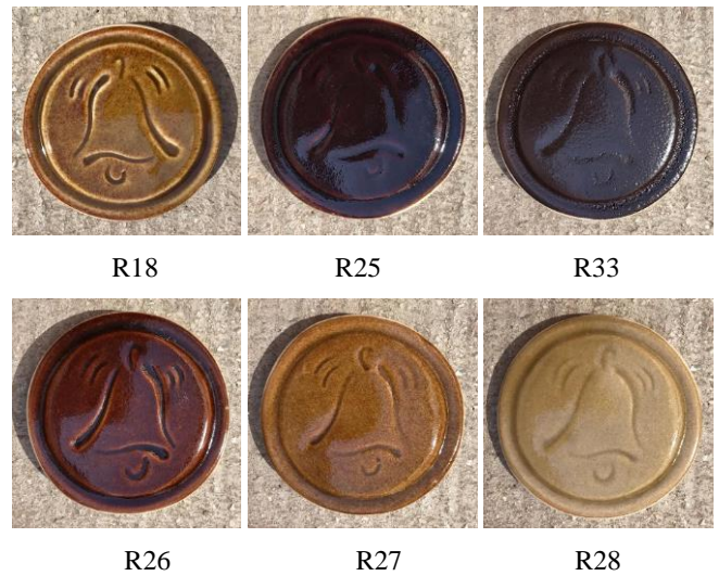
Figure 8. Surface images of glazes prepared with Çan stone waste after firing at 1200 °C (Diameter: 14 cm).
