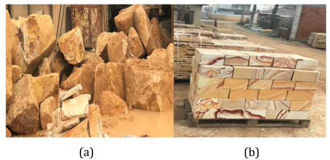
Figure 1. (a) Çan stones from the quarry, (b) Çan stone blocks cut in the factory.
