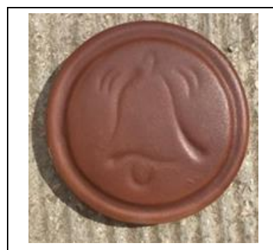
Figure 5. Appearance of Çan stone waste fired at 1200 °C.
