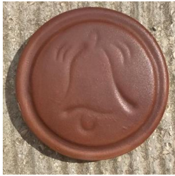
Figure 5. Appearance of Çan stone waste fired at 1200 °C
