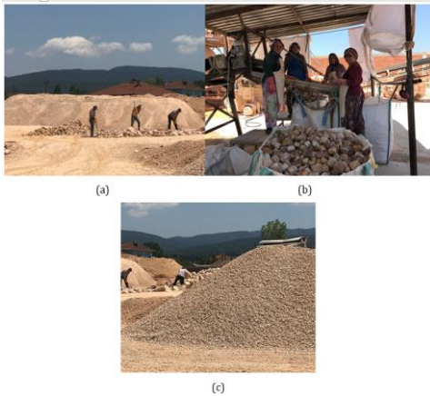
Figure 2. (a) Size reduction process with hammer (b) Tumbling process (c) Çan stone wastes after reduction.
